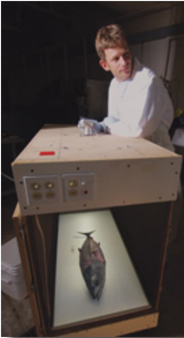
OSU faculty research assistant Sean Carroll photographs albacore tuna flesh in a "lightbox" to test different methods of handling fish to maintain the highest quality. Photo, Lynn Ketchum.
