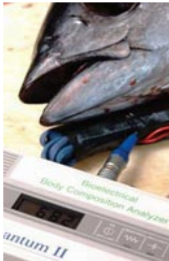
This device determines the body fat in albacore tuna, making it possible to sort fish by fat content for different markets. Photo, Lynn Ketchum
